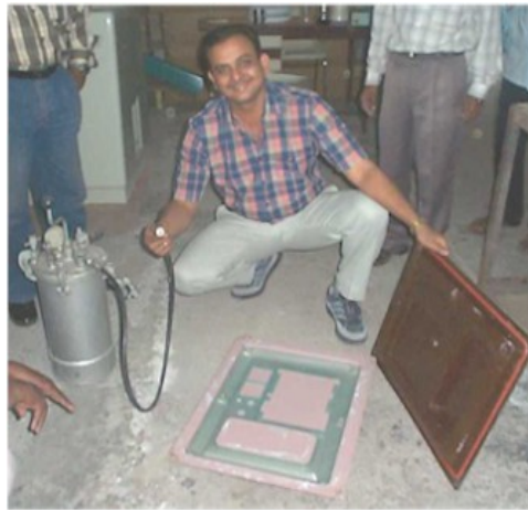
Miland Upasani CEO of ICE in Pune demonstrates their indigenously designed RTM process which is used to make machine covers. of very high quality.
