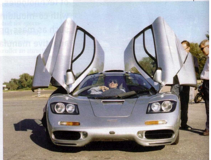
The author at the controls of the McLaren F1. This was the first automotive project to use advanced composites throughout. The industrial engineering philosophy made extensive use of statistics and measures of process capability.
