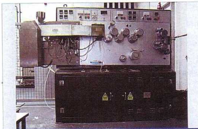
Fig. 3: Melt extruder for producing auxetic fibres at the University of Bolton, these are currently being converted for use in auxetic composites.
